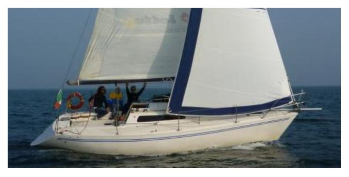
On this Stag 32 we installed our 70 mm anodized aluminum removable bowsprit that allowed us to exit from the bow without mounting an upwind.
