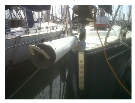
For the Salona 45 we made a custom bracket that had been studied for an extremely easy installation. The bracket is fixed to the bow's forestay heath thanks to a bolt. This one is sufficient to stop the bracket thanks to a specific milling that contains the heath.
