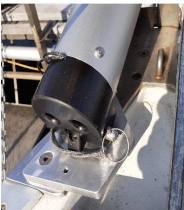
Stern fastening system with aluminum support plate
