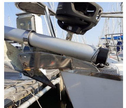
Detail of the ring bracket mounted inside the bow roller
