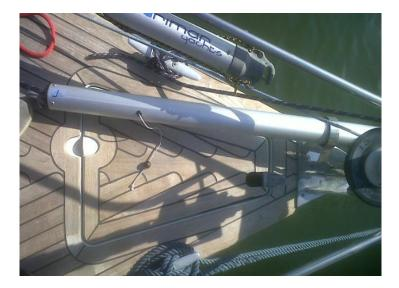
The Rimar 31.3 has a clear and clean bow that allows a quick installation of our removable bowsprit. It is mounted by using our standard angled bracket. The mounting was easy thanks to the clear access to the anchor's forepeak.
