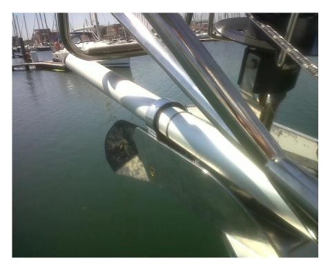
On this sailing boat we installed an aluminum anodized removable bowsprit with a diameter of 70 mm. We used an apposite bracket that had been studied for being easily mounted inside the bow nose. In addition, the bowsprit was strengthened with another tube to keep the tension that derives from the sailing boat tonnage as well as to contain the external profile diameter.
