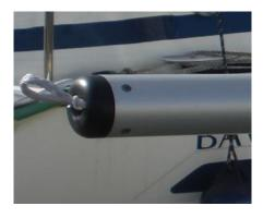
On the Oceanis 311 we installed an aluminum anodized removable bowsprit with a diameter of 70 mm. We used a bracket that had been studied for being easily mounted on the bow's nose side. Sail Service can install Dyneema ends for furling systems (see photos).
