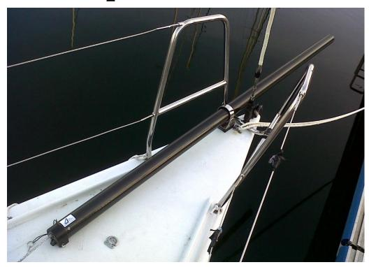
We installed our 70 mm removable carbon bowsprit on a racing monotype model "Lutra 30 v1". On this sailing boat, the installation was easier thanks to the absence of noses and anchors. It allowed us to use to mount our standard low bracket with a thickness to climb over the pulpit.
