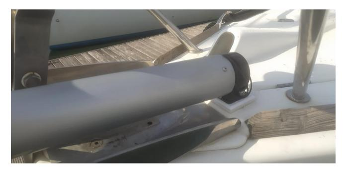
In this Jenneau Sun Odissey 36i, the bowsprit was installed in a way that the forepeak's entrance could stay clear. This way, the bowsprit could stay on even during a sailing cruise or when you would like to anchor.
