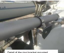
Detail of the ring bracket mounted inside the bow roller.
