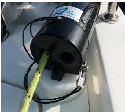
Stern fastening system with Delrin riser plate.
