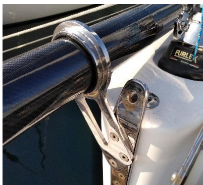
Ring bracket fixed with the screws of the mainsail (ORC regatta version).
