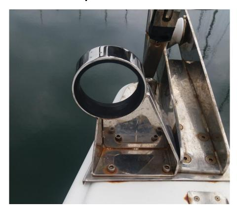
This GS 40 mounts the new version of the removable bowsprit with a more robust attachment. Just like the previous Grands Soleil's bowsprits, it had been created using an 80 mm tube that's fixed on the stern of the anchor locker.
