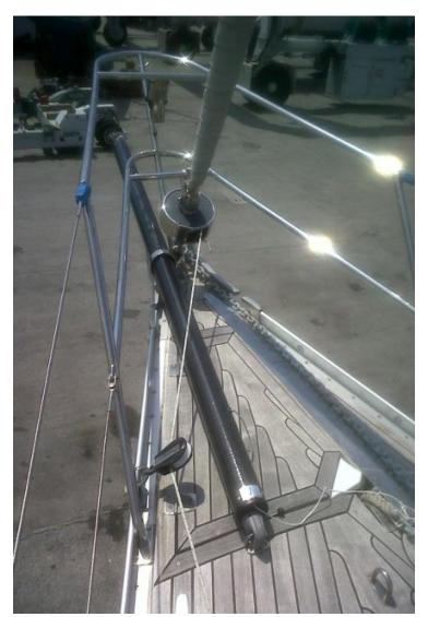
We easily installed the 80 mm carbon removable bowsprit on this Grand Soleil 39. To get rid of the bulkiness of the anchor snout, a standard 2 cm thick inclined bracket was used. The forepeak stays comfortable for the bracket as well as the pad eye bulks' fixing.
