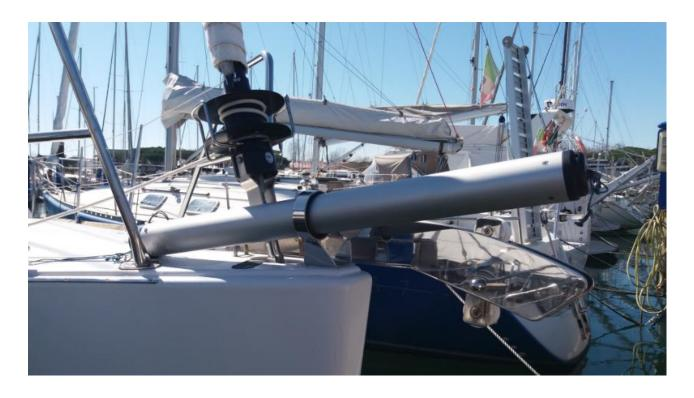
The Grand Soleil 37 mounts a standard kit of our new removable bowsprit. Here, we used our 80 mm bowsprit with inclined ring bracket. Although the overhang outside the bow does not go beyond the anchor nose, it can easily go out for a longer length. We did it only because the owner requested to do so.
