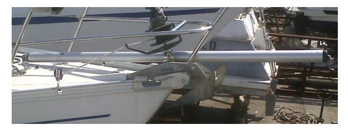
On this Grand Soleil 343 we installed our 80 mm aluminum removable bowsprit. Because we wanted to get rid of the anchor footprint, we decided to use a polyzene standard tall bracket with a thickness of 2 cm. The forepeak let the bow bracket's fixing while the fixing of the rear eyebolt had been made by passing through the bow's cabin and by opening a small compartment. In this installation, we preferred using the already existing of the fixed pad eye.
