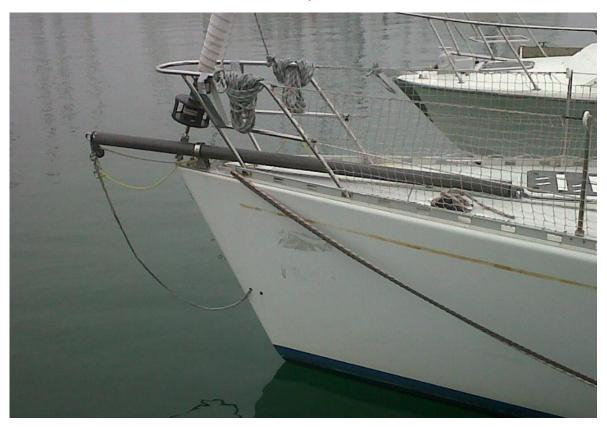
On this Este 39 we easily installed an 80 mm diameter carbon bowsprit with our standard tall bracket. The bracket is fixed on the stainless-steel bow nose; this way, the bracket stays clear from the overall dimensions of the bow pulpit and from the forestay. The bow forepeak allows an easy installation for both the pad eye and the bracket.
