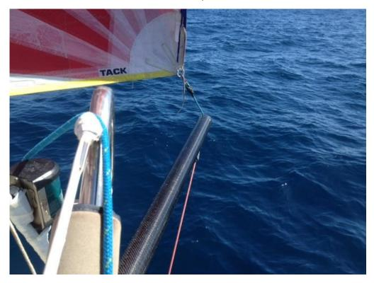
The owner of this Dehler 36 decided to install our carbon removable bowsprit by adding a rail that makes the pull-in-push-out easier. In fact, the action can be done by staying in the cockpit.
