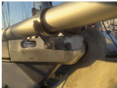
Ring bracket bolted directly to the bow roller.
