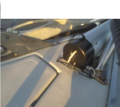
Stern fastening system with Delrin end and deck ring attached directly to the deck.
