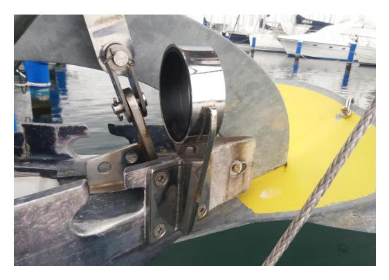
On this Comet 11, we installed our new 80 mm removable bowsprit in aluminum in a way that enables the forepeak's entrance clear.
