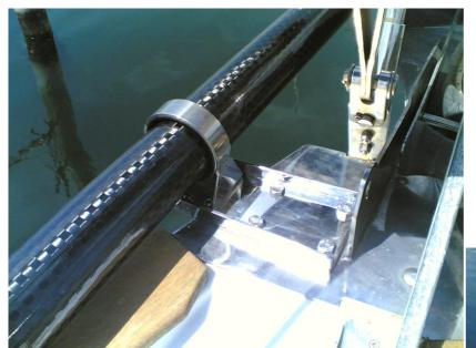
For this Bavaria 44', as we noted the important deployment, we chose a carbon bowsprit with an external diameter of 80 mm and a length of 2500mm. We made a special bracket, customely designed, disengage from anchor footprint. The foldable pad eye was set on the bow skylight.
